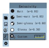
As shown in the figure, press "  $\oplus$ / MENU" key to enter the main menu and select "  $\mathcal E$  "(emissivity) option and press "  $\blacktriangleright$  " key to enter the emissivity list.
